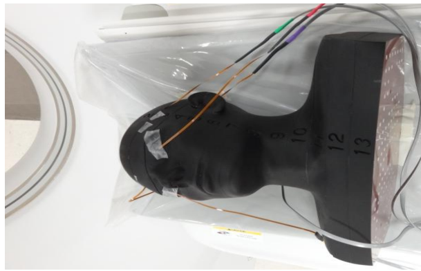
Figure 7: Anthropomorphic head phantom with dosimeters placed in the eye lens and brain regions
