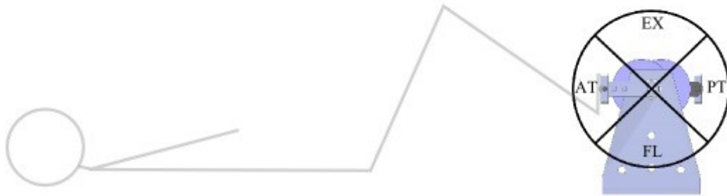
Figure 2.4 Quadrants of the pedaling cycle, anterior transition (AT), extension (EX), posterior transition (PT), and flexion (FL).
