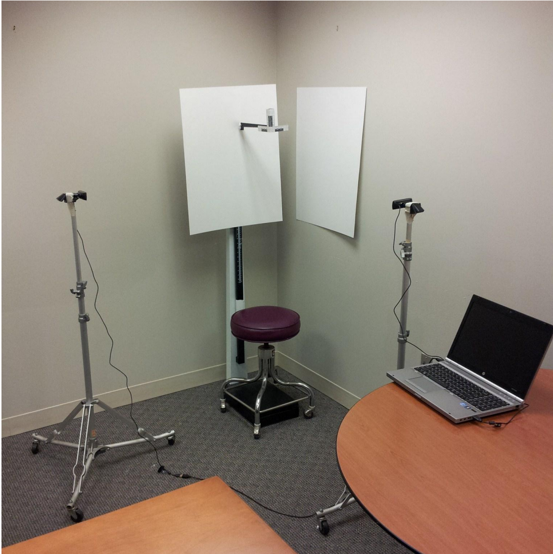
Fig. 1 Set-up for simultaneous frontal and right sagittal image capture with high-definition webcams
