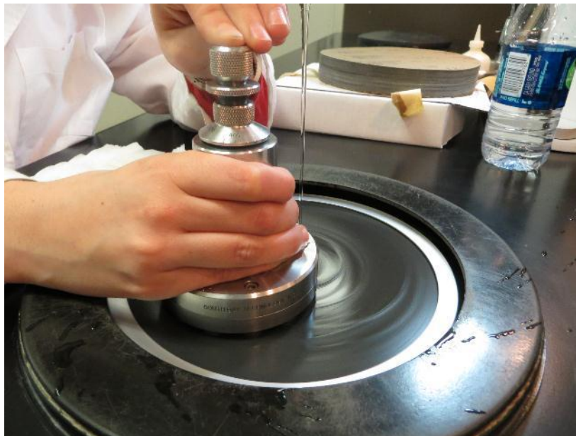
Figure 6. Grinding of specimens with silicon carbide paper to achieve 3 mm thickness after stain application.
