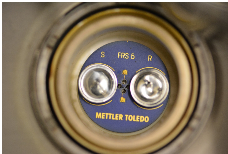
Figure 5: Aluminum crucibles on the sensor of the DSC. The crucible containing the file sample is on the left and the blank reference crucible is on the right.
