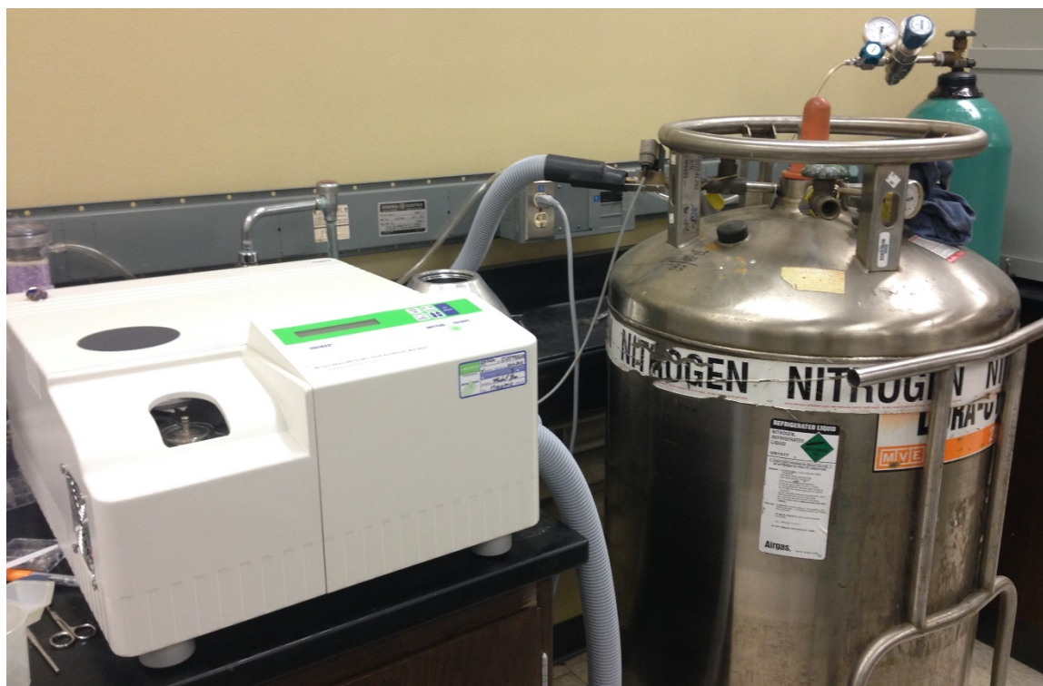
Figure 6: DSC equipment and liquid nitrogen.
