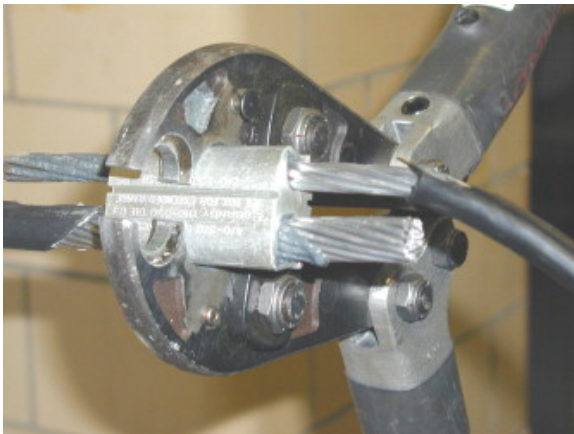
Fig. 1. An aluminum compression connector joining two cables. This photo shows the jaws of a Burndy MD6 enclosing the connector before the connector is pressed over the cables. When the connector is pressed, the aluminum deforms around the cables and makes an extremely tight connection.
