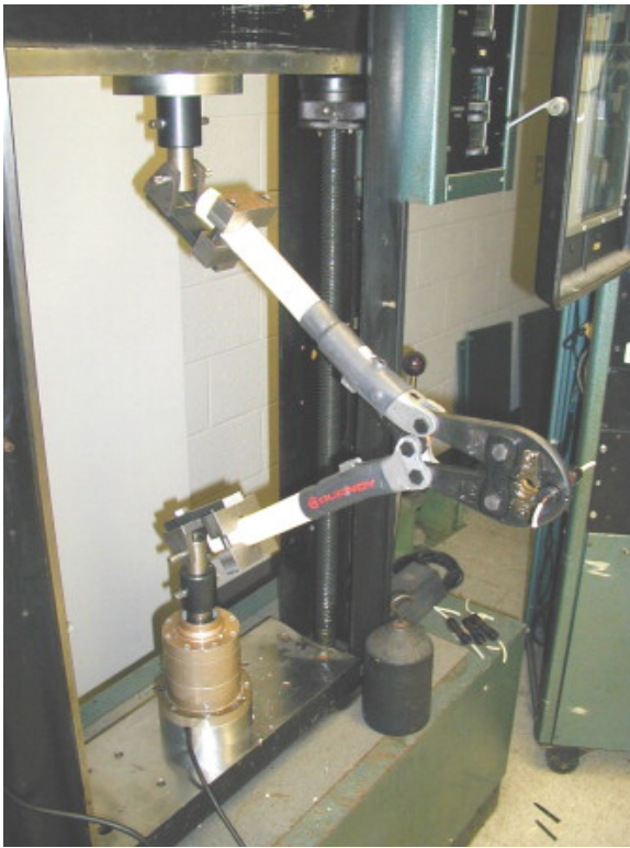
Fig. 6. Instron system applying vertical force to the handles of a manual press in order to crimp a connector. The drive cylinder is on the top, and the load cell is located at the bottom. Courtesy of EPRI (December 2001).
