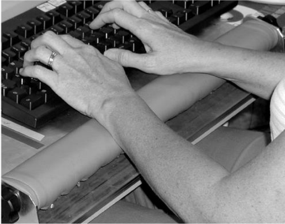
Figure 5. Keyboard force fixture with notebook computer and wrist support.
