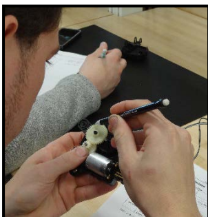
Figure 4: Counting gear teeth in HVAC baffle drive in Experiment 4.
