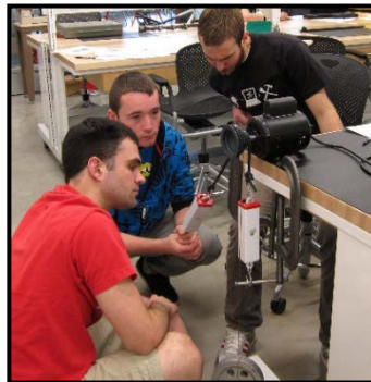
Figure 6: Investigating belt tension in Experiment 5.
