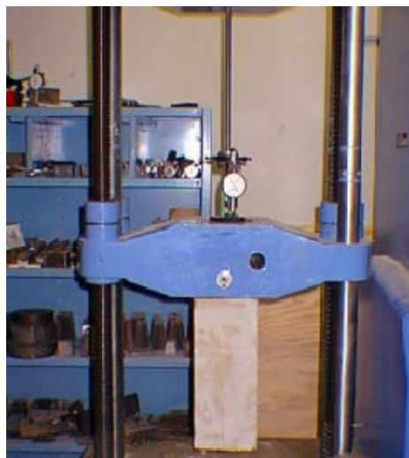
Figure 2.3.2 Pull-Out Test Set-up
