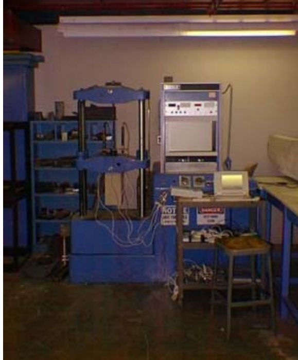
Figure 2.4.1: Modified Pull-Out Test Set-Up
