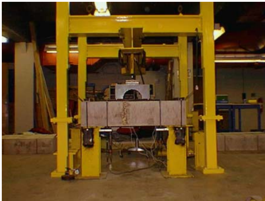
Figure 2.2.2: Joint Deflection Test Set-up
