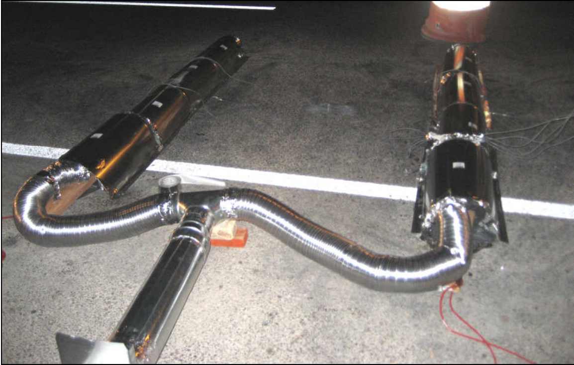
Figure 2-17 - The heating assembly was placed over the two slots cut for the WIM sensors. Heat was supplied by a forced-air kerosene fueled heater (not pictured). The sections of the assembly were sealed with aluminum ducting tape to minimize heat loss. Multiple temperature probes were in place to accurately measure pavement temperatures.
