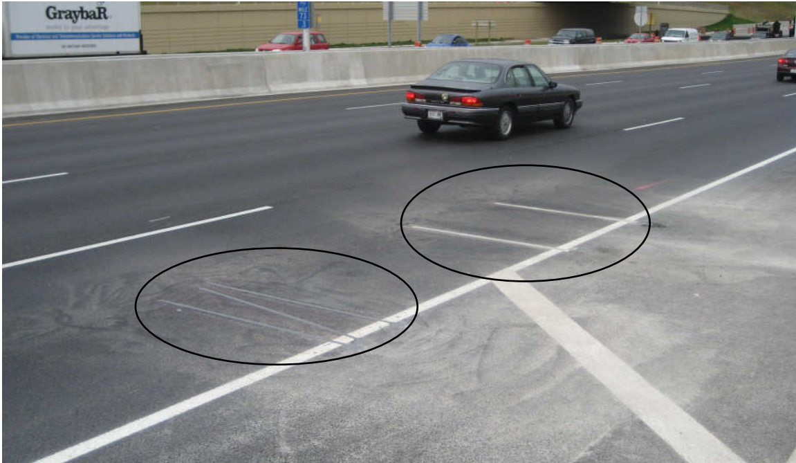
Figure 2-19 – Test section opened to traffic with the wheel-wander and WIM sensors installed (circled areas).
