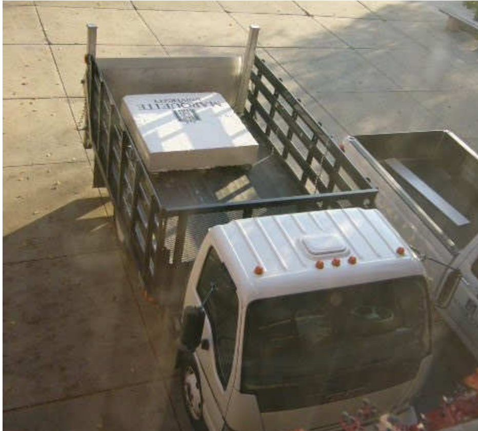
Figure 2-20 - Vehicle used to calibrate the WIM system. Note the concrete slab placed in the bed of the truck over the rear axle.
