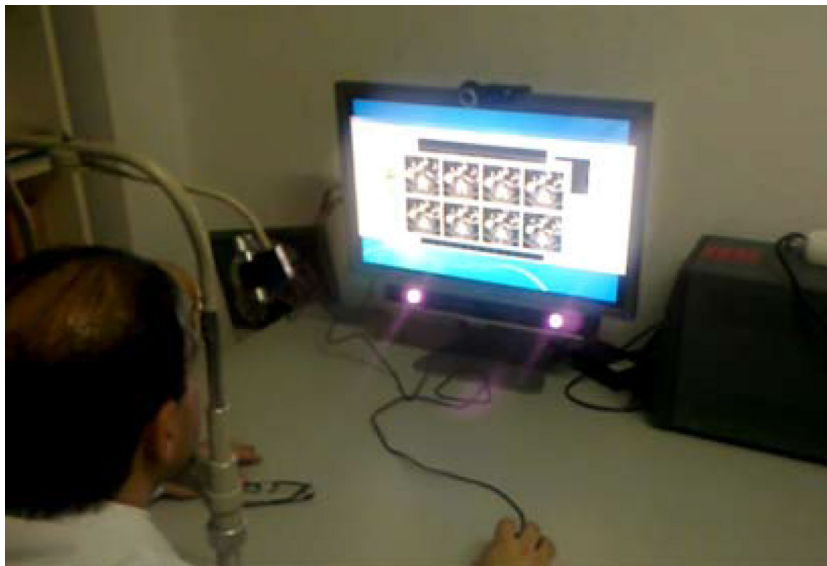
Figure 2 Surgeon using the early version of the SI. The SMI eye-tracker is visible below the monitor.
