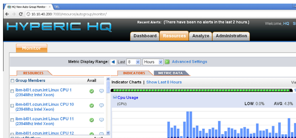
Fig. 12. Overall (or per process) CPU, memory network and other resource usages can be tracked with Hyperic for cloud service accounting.
