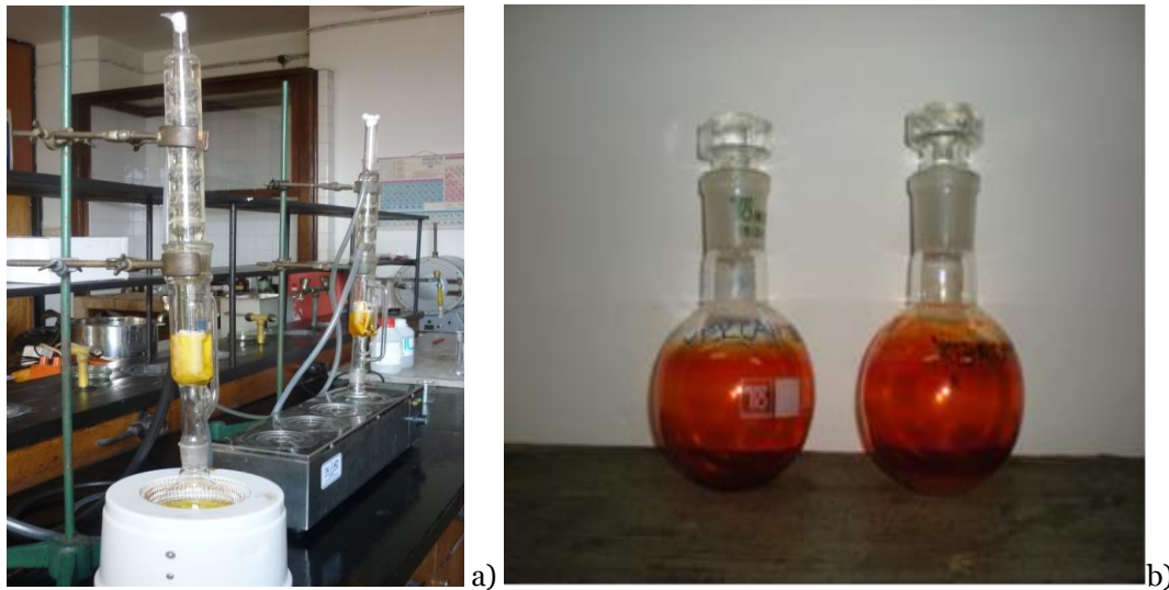
Fig. 4.3. Extraction of red hot pepper by Soxhlet procedure (a), and obtained extract (b).
