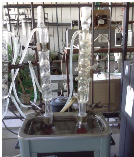
Fig. 4.2. Ultrasound extraction of red hot pepper.
