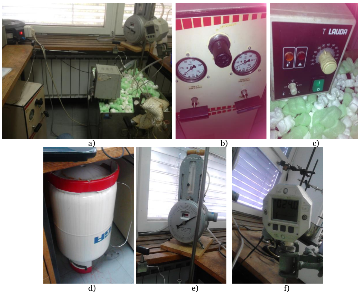
Fig. 4.6. System for extraction with dense propane (a): high pressure pump (b), regulator and temperature indicator (c) gas bottle (d), rotameter (e) and pressure indicator (f).
