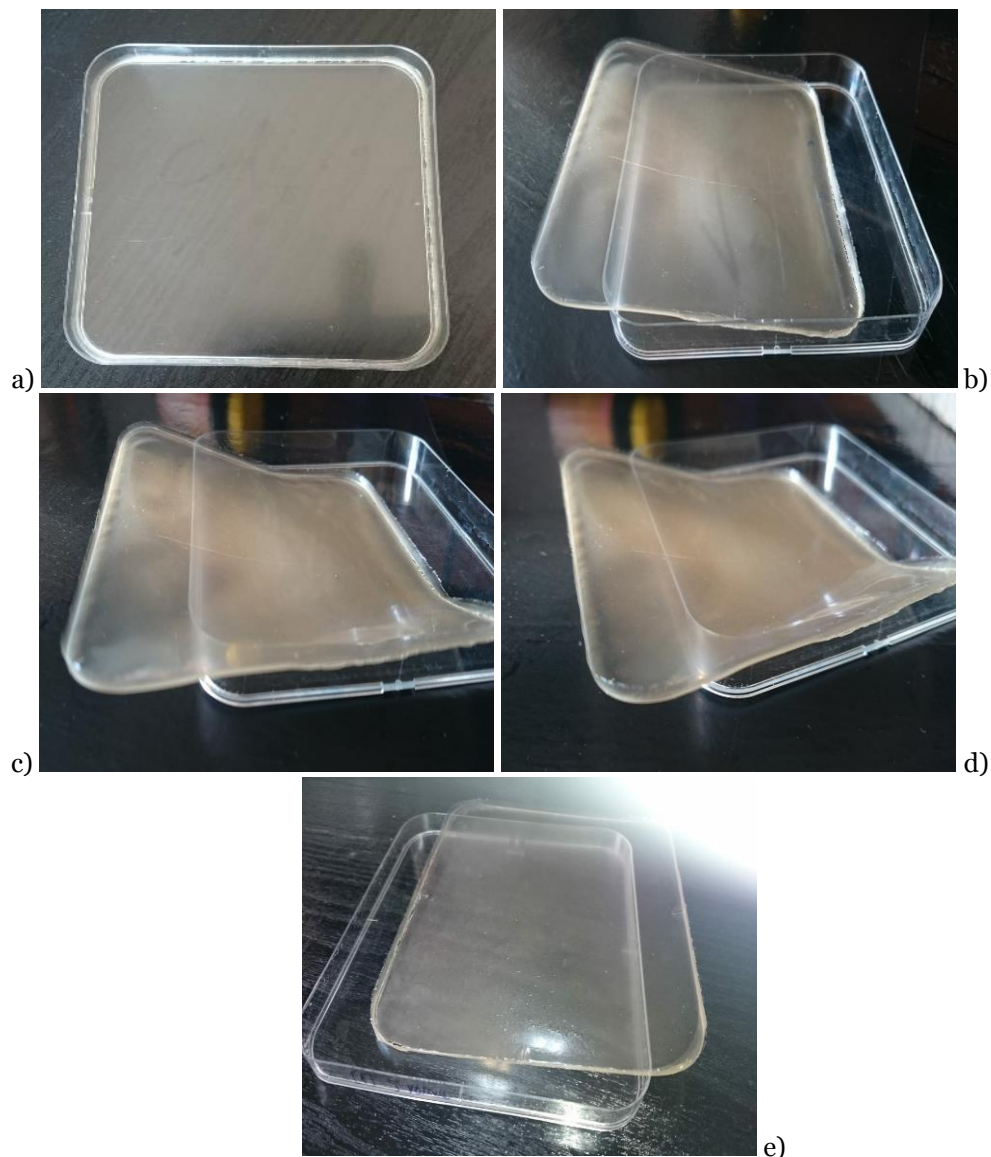
Fig. 5.19. Appearance of the edible films with different quantity of seed extract of red hot pepper: (a) 10 mg-S 10 ; (b) 20mg-S 20 ; (c) 30 mg-S 30 ; (d) 50 mg-S 50 and (e) 100 mg-S 100 .
