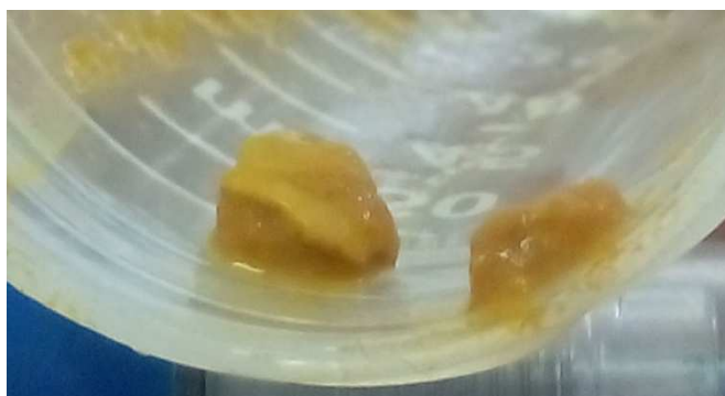
figure 28: stratification of the solid residue after centrifugation
