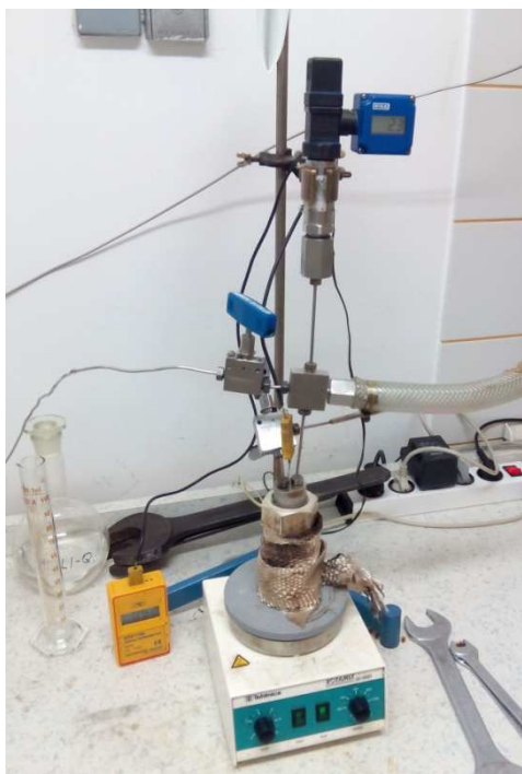
figure 16: autoclave used in the experiments
