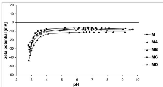
(M-Modal fibre, MA-nanocoated Modal fibres by using procedure A, MB- nanocoated Modal fibres by using procedure B, MC- nanocoated modal fibres by using procedure C, MD- nanocoated Modal fibres by using procedure D)
