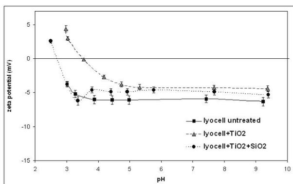
(untreated Lyocell fibres,  $\text{TiO}_2$  nanocoated Lyocell fibres and  $\text{TiO}_2\text{-SiO}_2$  nanocoated Lyocell fibres)
