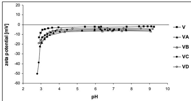
(V-Viscose fibre, VA-nanocoated Viscose fibres by using procedure A, VB- nanocoated Viscose fibres by using procedure B, VC- nanocoated Viscose fibres by using procedure C, VD- nanocoated Viscose fibres by using procedure D)
