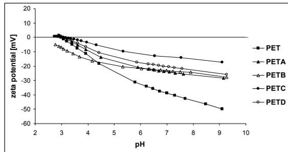
(PET-polyethylene terephthalate fibre, PETA-nanocoated polyethylene terephthalate fibres by using procedure A, PETB- nanocoated polyethylene terephthalate fibres by using procedure B, PETC- nanocoated polyethylene terephthalate fibres by using procedure C, PETD- nanocoated polyethylene terephthalate fibres by using procedure D)
