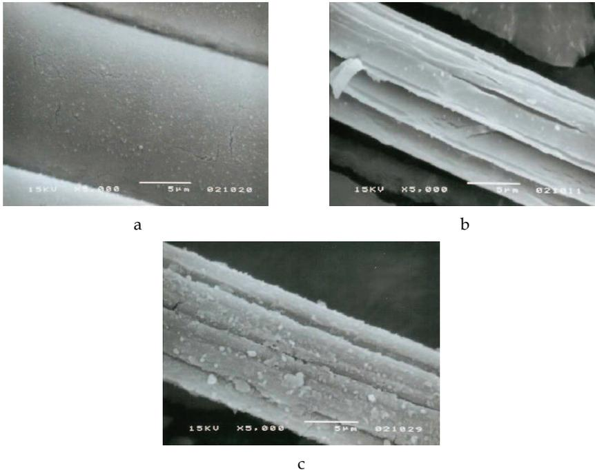
Fig. 2. SiO<sub>2</sub> nanocoated PET fibres (a) and regenerated cellulose fibres Modal (b) and Viscose (c) according to the procedure B
