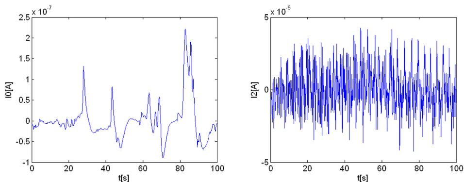
Fig. 1. Current noise signal corresponding to: a) X5CrNiMo17-13 stainless steel in borate buffer solution + 0.1 mol/dm<sup>3</sup> NaCl at the passive potential ( $I_0$ ); b) Low Carbon Steel in 0.1mol/dm<sup>3</sup> H<sub>2</sub>SO<sub>4</sub> at the corrosion potential ( $I_2$ ) (Planinšič & Petek, 2008).
