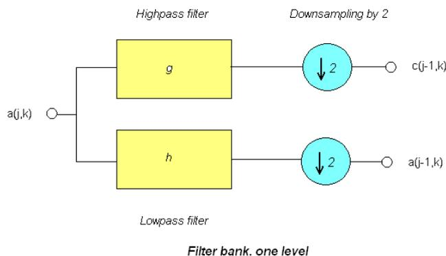
Fig. 5. One stage of analysis filter bank
