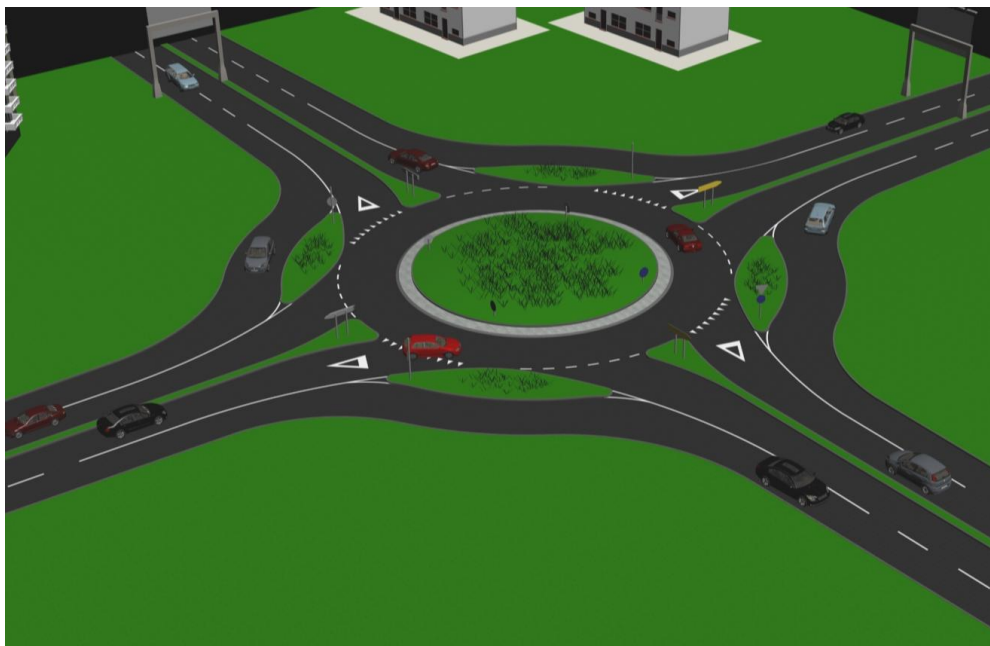
Figure 6 - The roundabout with "depressed" lanes for right-turners
