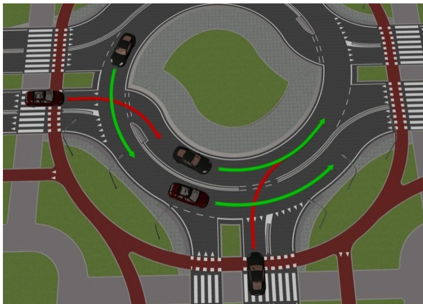
Figure 5 - Crossing conflict point at the entry on the inner circulatory carriageway from the inner lane at the entry
