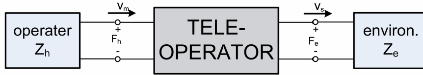
Figure 2. Network model of a bilateral teleoperation system
