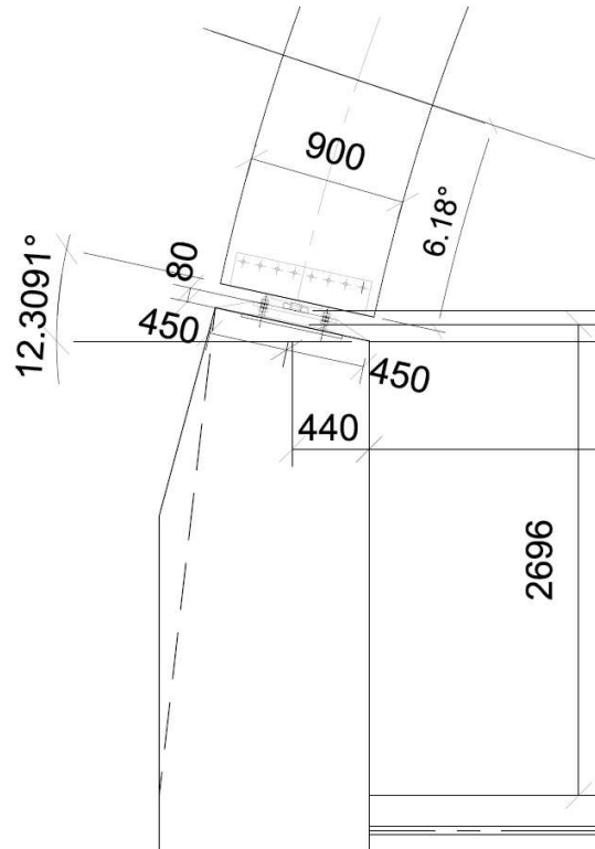
Fig. 10 Detail of the foot base of the arch timber truss with foundation structure
