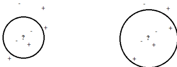
Figure 2.4: Classifying a new instance with k-nearest neighbours for k=3 (left) and k=5 (right).
