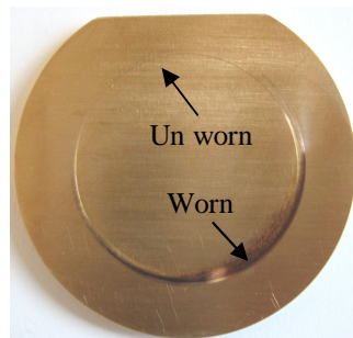
Figure 6.4 Worn-unworn areas on test disc in TWT apparatus 1.
