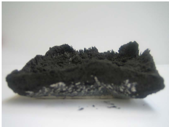
Figure 15. 450CA30 Cone Calorimeter Sample Intumescence
