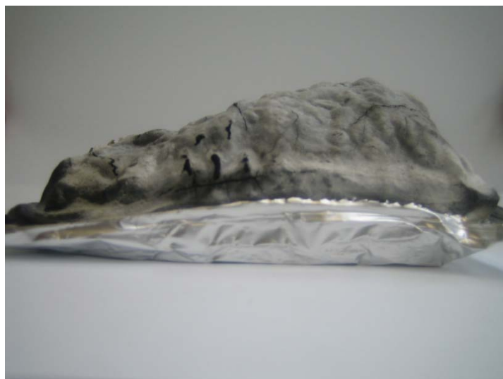
Figure 14. 450GL30 Cone Calorimeter Sample Intumescence
