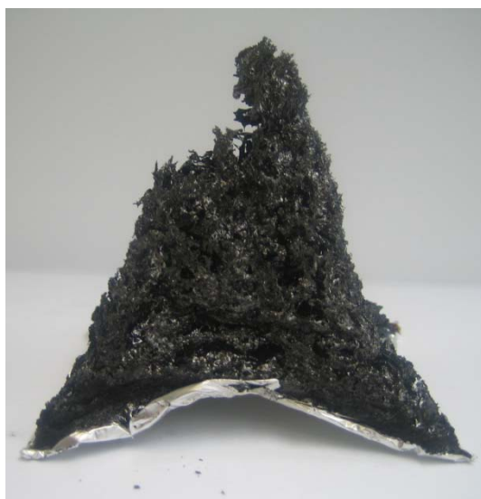
Figure 13. 450G Cone Calorimeter Sample Intumescence
