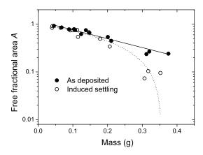
Figure 2: Reduction in the free fractional area of a glass slide with increasing quantities of sand. Filled circles show the as-deposited coverage while open circles show coverage after application of gentle disturbance to the glass slide. The solid and dotted lines are exponential and linear fits to the data respectively.
