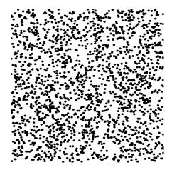
Figure 4: A Monte Carlo approach was used to simulate particle accumulation on PV modules. The figure shows an example image obtained for n=2000 particles. Images were obtained for other values of n and subsequently analysed.
