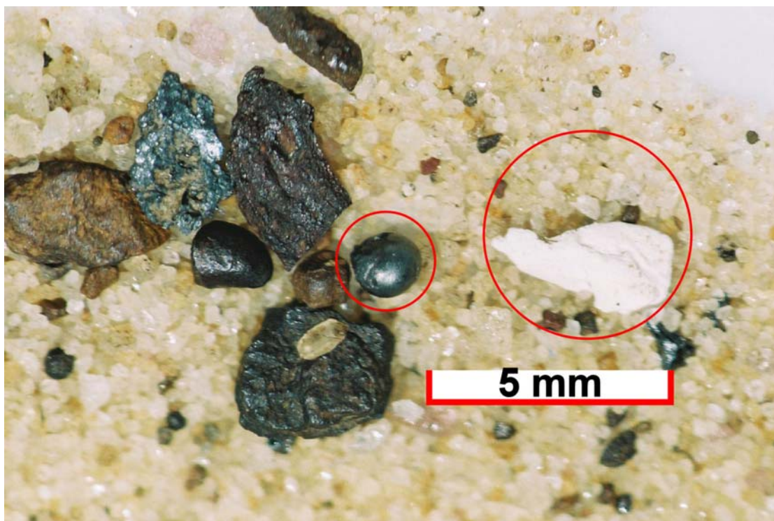
Photograph 1: Anthropogenic contamination observed in some G-BASE panned heavy mineral concentrates. Top – Sample 307349P showing oxidised lead shot. Bottom – Sample 307364P showing steel shot and a flake of paint.
