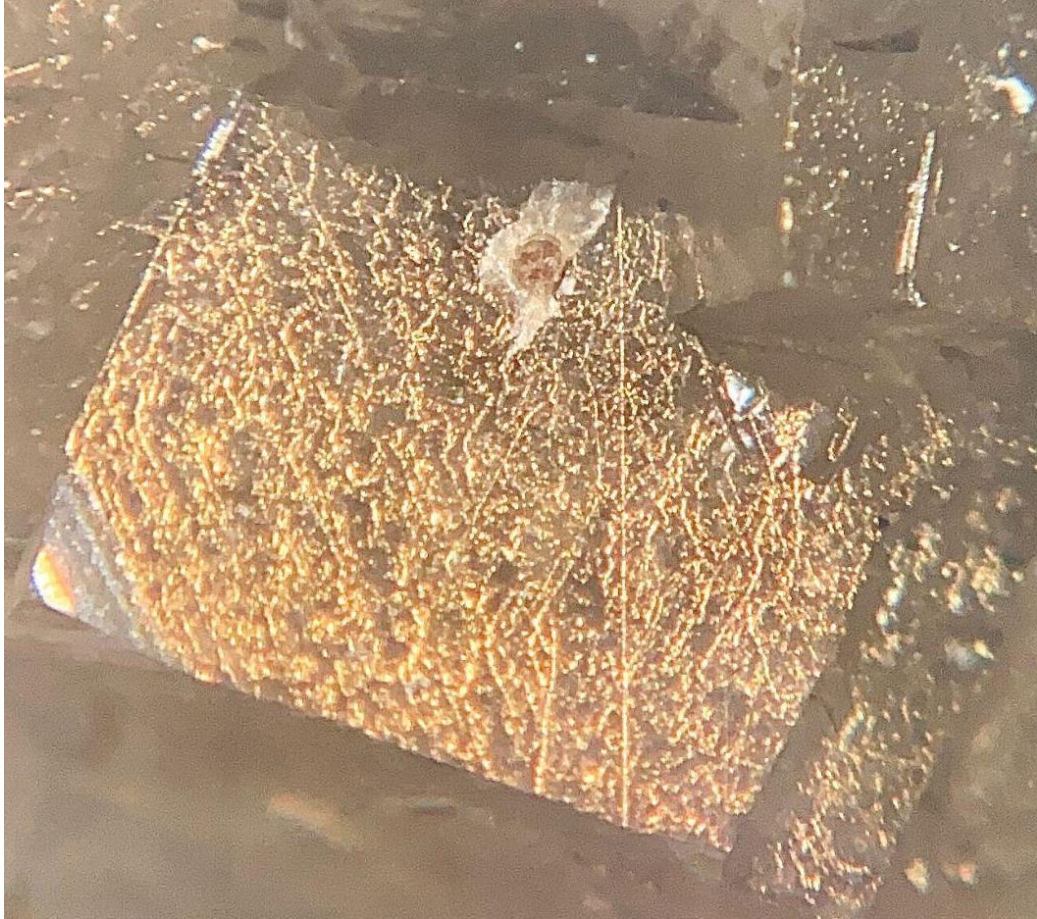
Figure 26: Angular and straight-line texture on the surface of a primary rhombohedron.
