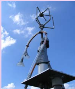
Fig. 1 Arrangement of the inlet lines close to the ultrasonic anemometer (PTFE for the gases: N 2 O, CO 2 , H 2 O, VOCs, copper tube for aerosols).
