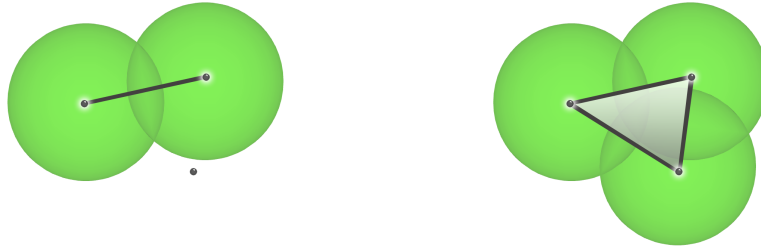
■ Figure 1 The nerve has an edge for each pairwise intersection, a triangle for each 3-way intersection (right), etc.
