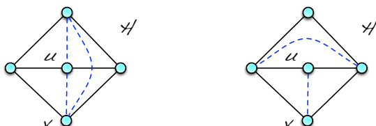
■ Figure 1 In the instance of k -LS-FI, k = 3 , the original edges of G = (V, E) are solid lines, and the fill edges F are dashed lines. Graph H = (V, E \cup F) is one of two minimal triangulations of G = (V, E) and H' on the right side is a solution of the provided 3-LS-FI instance. However, graph H' is not a minimal triangulation of G as H' \setminus uv is chordal and to obtain a minimal triangulation H' \setminus uv from H one has to swap four edges.
