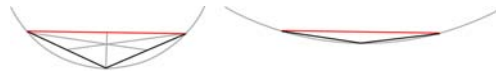
■ Figure 8 Circumradius of the triangle adjacent to the boundary edge (red) increases after particle insertion, as the boundary edge cannot be flipped to produce better conditioned triangles. Such cases are avoided by splitting of boundary edges.
