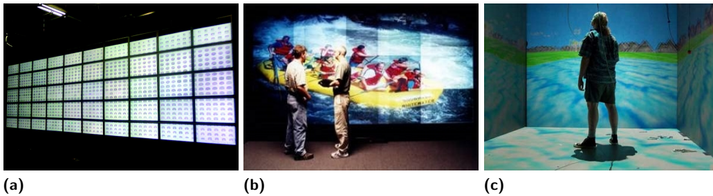
■ Figure 1 Possible large high-resolution display configurations: (a) monitor-based tiled display wall, (b) projector-based tiled display wall, (c) Cave Automatic Virtual Environment (CAVE TM ).
