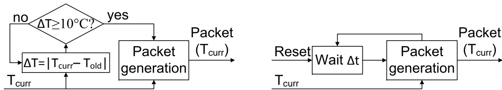
■ Figure 1 (a) Event-driven and (b) Time-driven temperature forwarding
