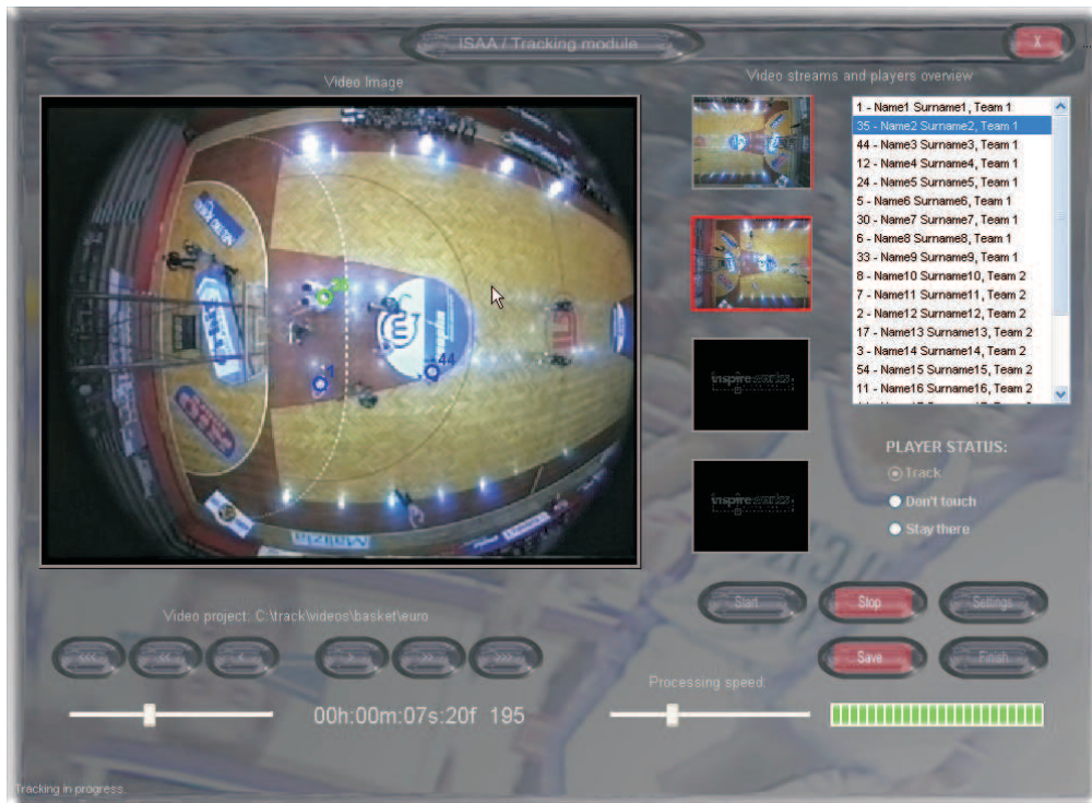
Figure 4: User interface of the tracking module. Three players are marked for tracking, one of them is "in focus" - selected in the player list on the right side and marked with green circle.
