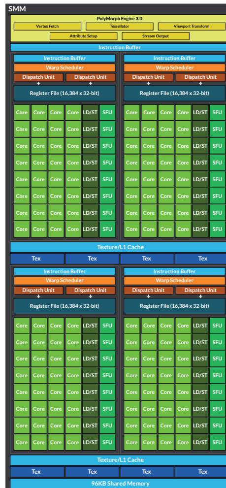
Figure 3.12: GM204 SMM Diagram (GM204 also features 4 DP units per SMM, which are not depicted on this diagram). NVIDIA Corporation [41, pg. 08]
