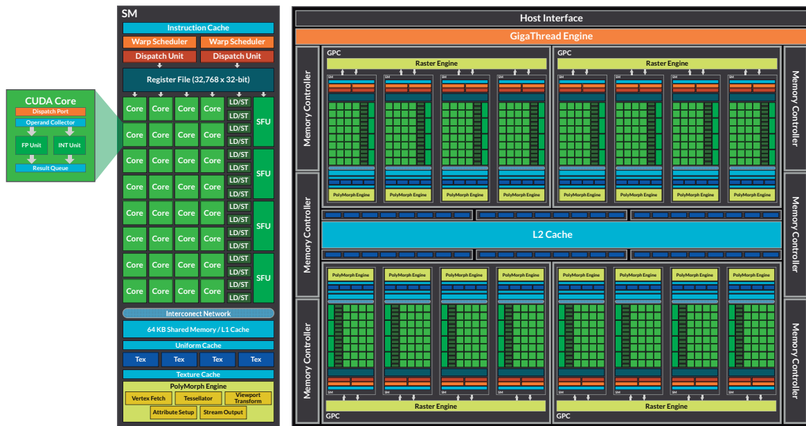
Figure 3.6: GF100 block diagram and Stream Multiprocessor detail. [31, pg. 11 and 16]
