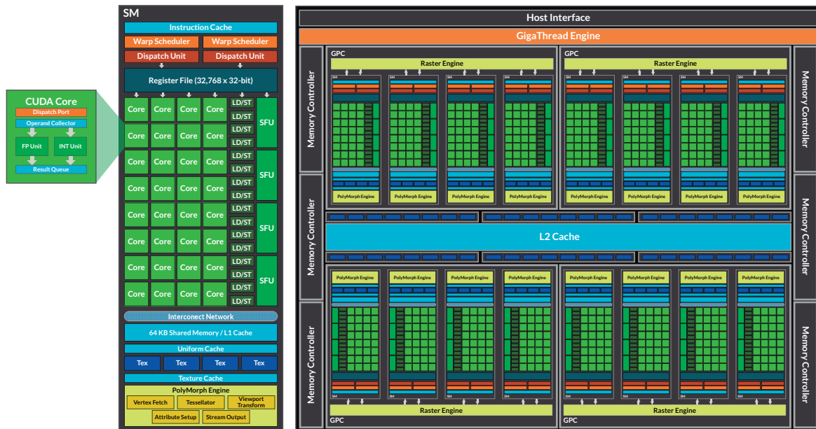
Figure 3.6: GF100 block diagram and Stream Multiprocessor detail [11, pg. 11 and 16].
