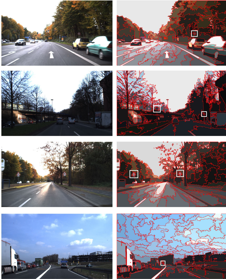
Figure 5.12: (Left) Examples from the GTSD dataset; and (right) layers of the hierarchy where traffic signs are detected (marked with white squares).
