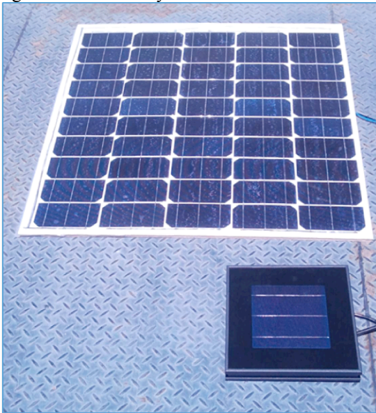
Figure 5: Module 1 and calibrated photovoltaic reference cell
