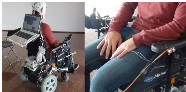
Figure: Robotic wheelchair controlled by the BCI system
