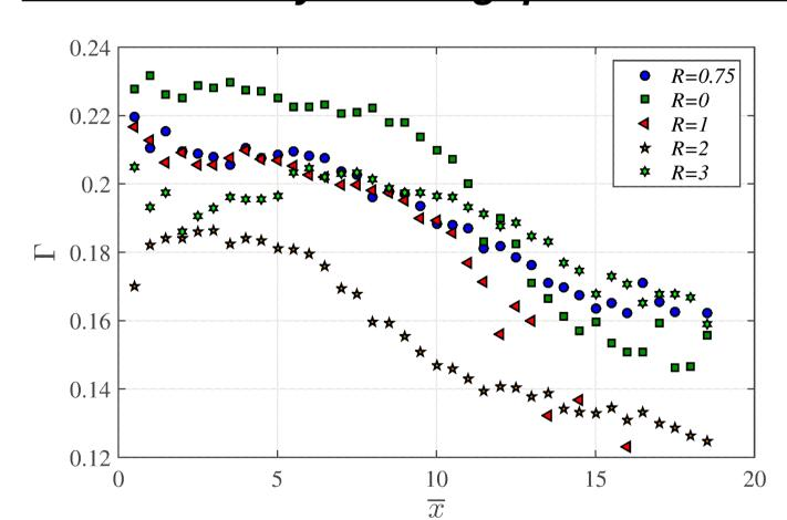
The continuous jet is a powerful tool to destroy the wingtip vortex for R greater than 1.
