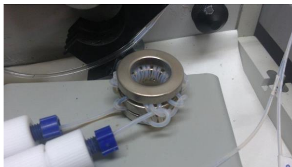
Figure 1. Knotted reactor to a Nd magnet as a sandwich between other two Nd magnets
