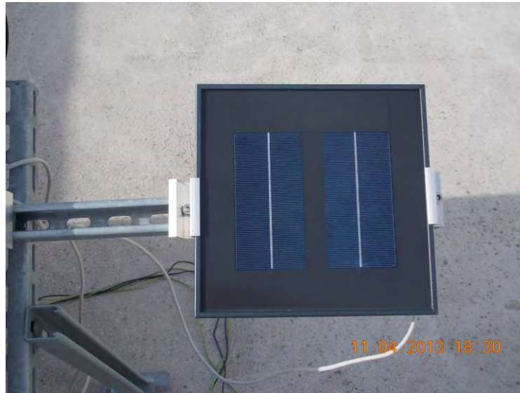
Figure 6.4. EPS PV Lab test bench incident irradiance monitoring calibrated cell detail.
