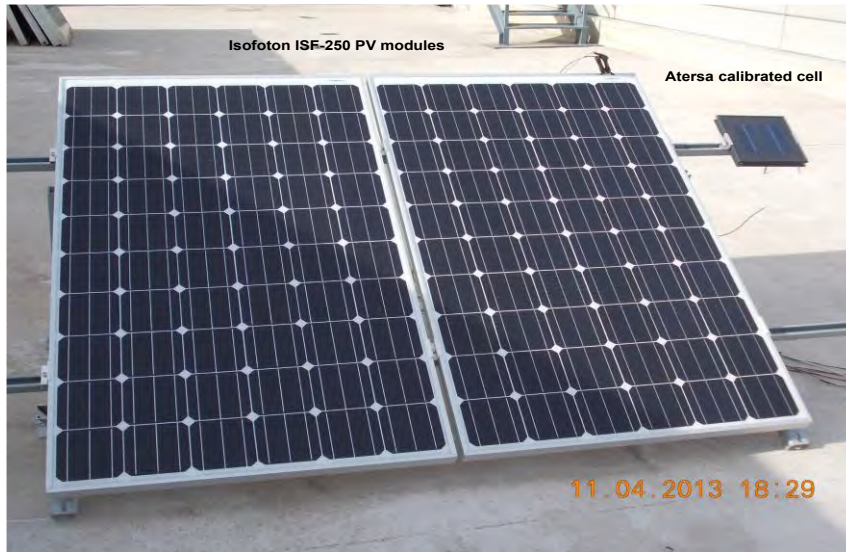
Figure 6.2. EPS PV Lab test bench PV module and calibrated cell assembly Test Bench structure
