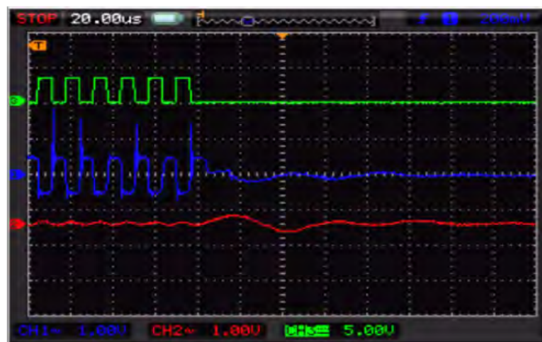
Figure 3.26. Test bench signals. Square signal by \mu Controller (CH1). Received signal at the end of the PLC line (CH2). DC signal at the inverters input (AC filtered)(CH3)
