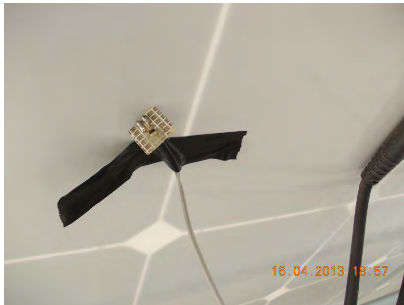
Figure 6.3. EPS PV Lab PV module back-plane temperature measurement with PT100 RTD
