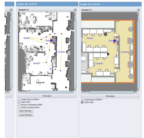
Fig. 2. From left to right, the geometrical, topological, and schematic maps of the test environment, embedded into the implemented plugin. Only the later one is shown to the subjects of our evaluation.
