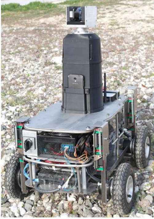
Fig. 8. The 3D laser scanner mounted on the outdoor mobile robot Andabata.
