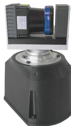
Fig. 1. The new 3D rangefinder UNOmotion for mobile robotics.
