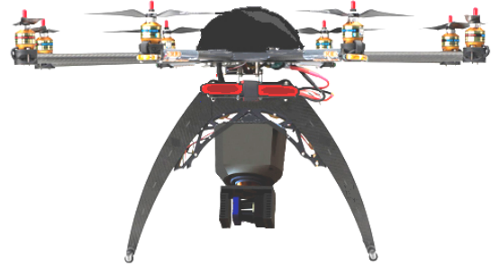
Fig. 7. Illustration of UAV sensor mounting.
