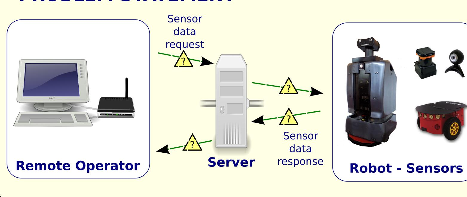
Stochastic transmision times prevent proper execution of some real-time control tasks (e.g. navigation)
