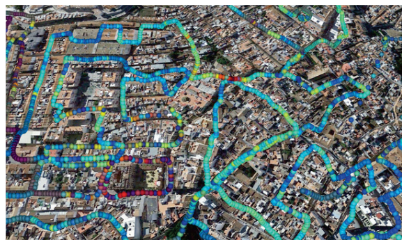
Figure 5. Spatial representation of the e-nose data collected during the inspection of an urban area. A jet color scale is used to represent the measured gas concentration.
