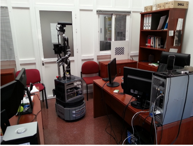
Figure 5. Mobile robot Rhodon gathering 3D data from an office.
