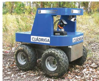
Fig. 4. Quadriga mobile robot with onboard 3D rangefinder.
