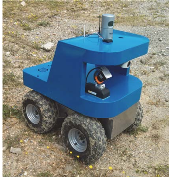
Figure 3. The Quadriga mobile robot with the HDL-32E sensor mounted on top.
