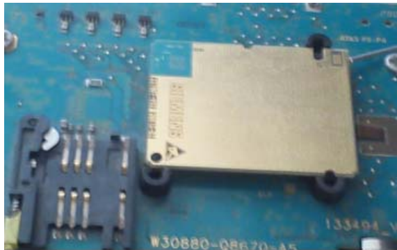
Figure 5: Telemetry electronic system: TC-65i.
