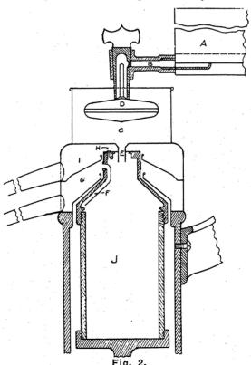
Vertical section of a cream separator bowl without inside fixtures.
