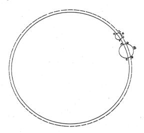
resents a horizontal section of a skim-milk tube and a cream tube of a machine of the type of the Empire at a point just before the respective products are discharged from the bowl.
