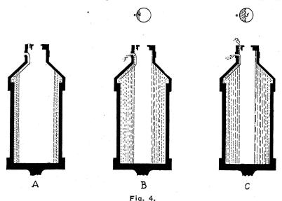
Vertical section of a separator bowl. Shows method of discharging skim-milk and cream.
