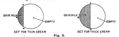
Cross section of skim-milk tube, separator set for thin and thick cream.
