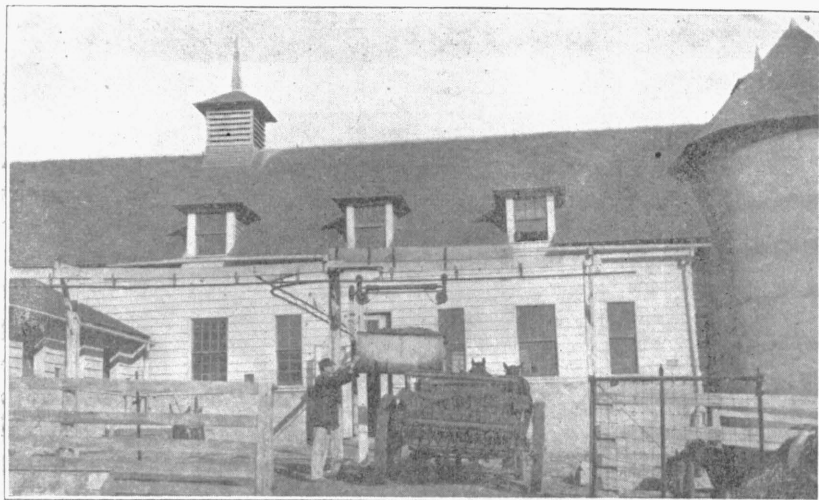
Fig. 7.—Litter carrier for dairy farm. The manure is collected in the carrier and dumped directly into the spreader.
